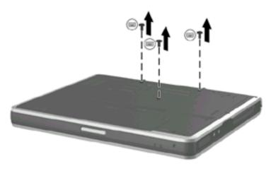
Removing the keyboard screws
